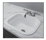
**General:** Furnish and install as shown on plans, an Undermount sink model 2218 as manufactured by E. L. Mustee & Sons, Inc. Material composition shall be molded fiberglass, using matched metal molds under extreme heat and pressure. One-piece, seamless construction with self-rimming edge for Undermount or top mount installation. Shall meet ANSI Specification Z 124-2017. Overall size 18" length x 22" width x 11" depth, weight 16 lbs., Color: White.
